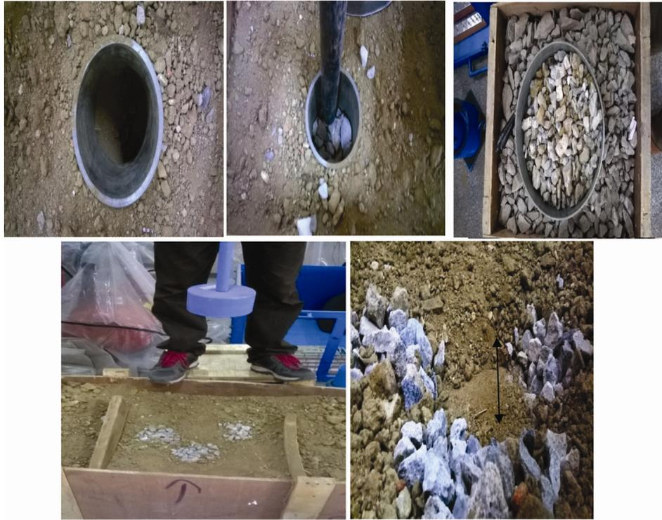
**Figure 8.** Broad experimental demonstration of reinforced demolished concrete waste as stone column.
