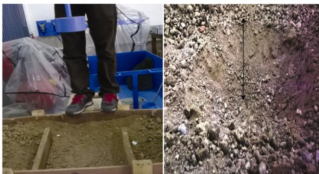
**Figure 7.** Broad experimental demonstration of impact loading on loose fill soil.
