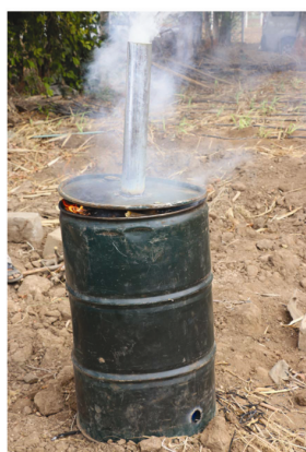
Figure 1. The chimney welded onto the lid of the outer drum.
