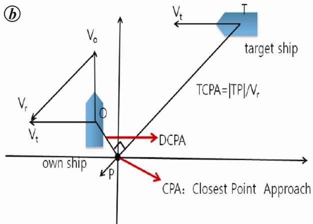
**Figure 2.** a, Sample leg with coordinates  $(x_1, y_1)$ ,  $(x_2, y_2)$ ,  $(x_3, y_3)$  and  $(x_4, y_4)$ . b, DCPA and TCPA between two vessels.
