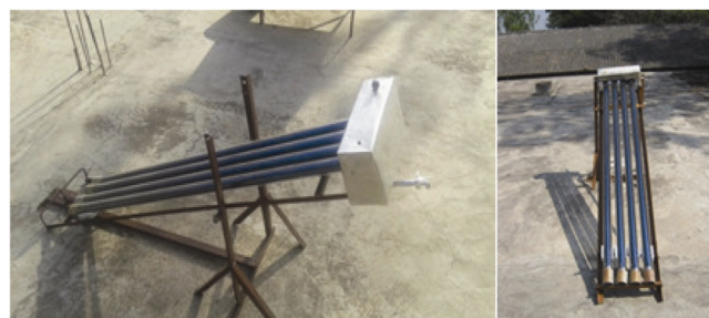
Figure 1. Four-tube solar water purifier.
