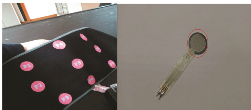
Figure 1. Sensor positioning on the belt and the sensor used. The positions represents abdominal regions, right hypochondriac, right lumbar, right iliac, epigastria, umbilical, hypo gastric, left iliac, left lumbar and left hypochondriac.
