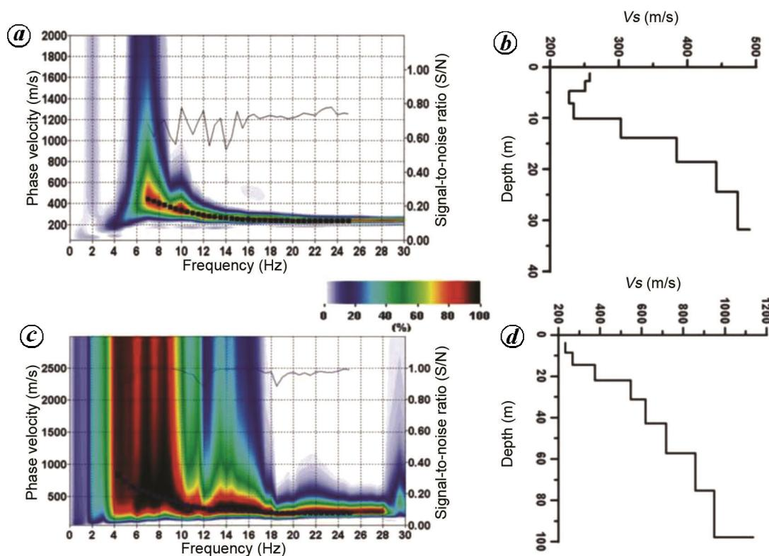
Figure 2. Dispersion curves and their corresponding one-dimensional shear wave velocity profiles.
