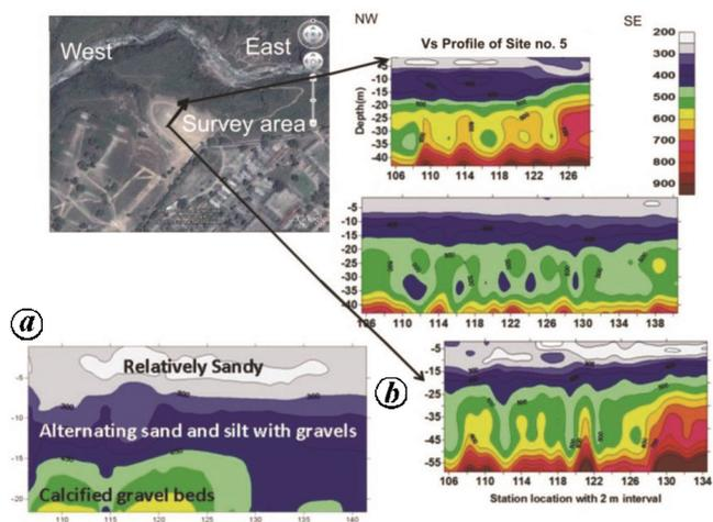
**Figure 5.** a, Correlation of upper 20 m soil column of Anarwala site with the field investigations for characterization of lithounits. b. The shear wave velocity profiles of Anarwala, site no. 5 along three parallel west to east running profiles to represent the alignment of palaeo-channels. The Google photograph (upper left) shows the location of the ground covered under the study and arrow represents the direction of palaeo-channel.
