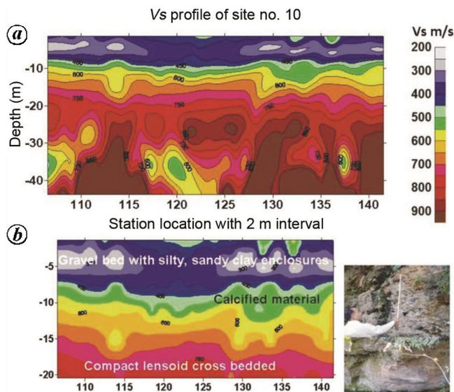
**Figure 6.** a, Shear wave velocity profile of Birpur site no. 10 (zone 2), which shows a low shear wave zones beneath station location 109–110 and 118–124. b, A blow up of top 20 m soil column, which has been measured and correlated with the field investigation.
