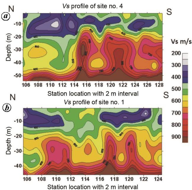
**Figure 3.** *a*, Shear wave velocity profile of Malsi Dear Park, site 4 (zone-1), showing almost vertical contact between Older Dun Gravels and Middle Siwalik Sandstone at a depth of 20 m below 114 station number. *b*, Shear wave velocity profiles of Shehanshai Ashram, site 1 (zone-1).
