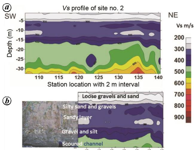
**Figure 4.** *a*, Shear wave velocity profile at SPRR, site no. 2. Reversal of shear wave velocity is noticed at a depth of about 10 m. *b*, shows comparison of  $V_s$  with lithology.
