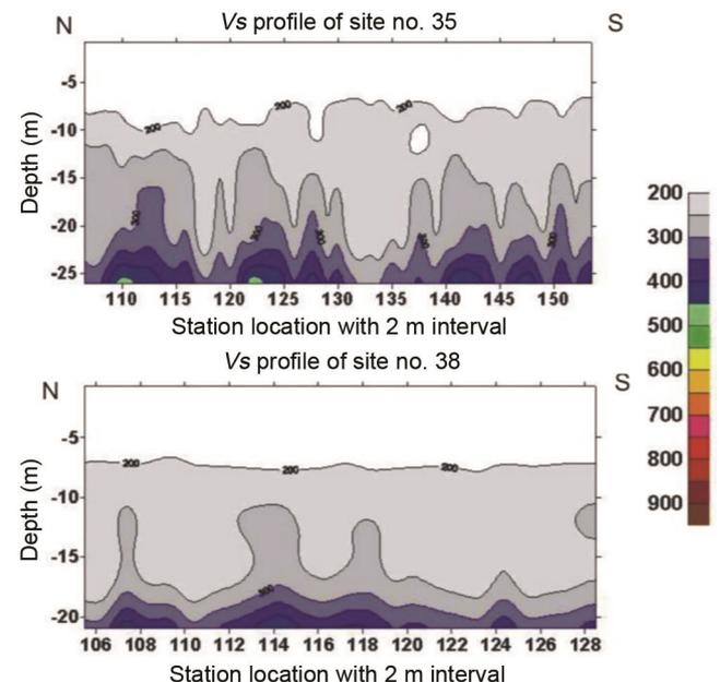
**Figure 8.** Shear wave velocity profiles of site nos. 35 and 38 (zone 4), showing the thickness of low clay deposits (~200 m/s).
