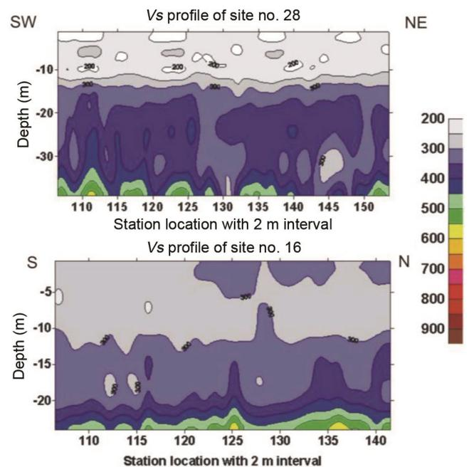
**Figure 7.** Shear wave velocity profiles of site nos. 28 and 16 (zone 3) showing the depth of low shear wave velocity sediments (~300 m/s).
