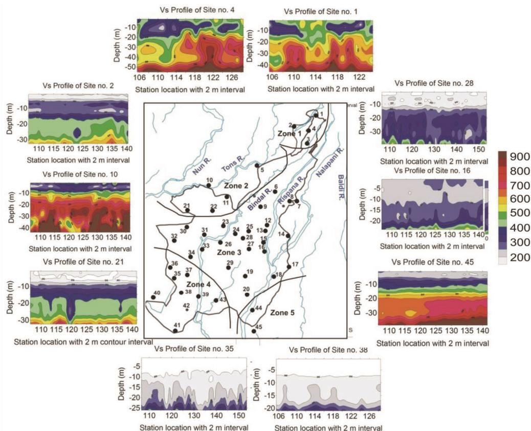
**Figure 10.** Classification of Dehradun Fan sediments in different zones based on shear wave velocity information of the subsurface up to 40–50 m depth.
