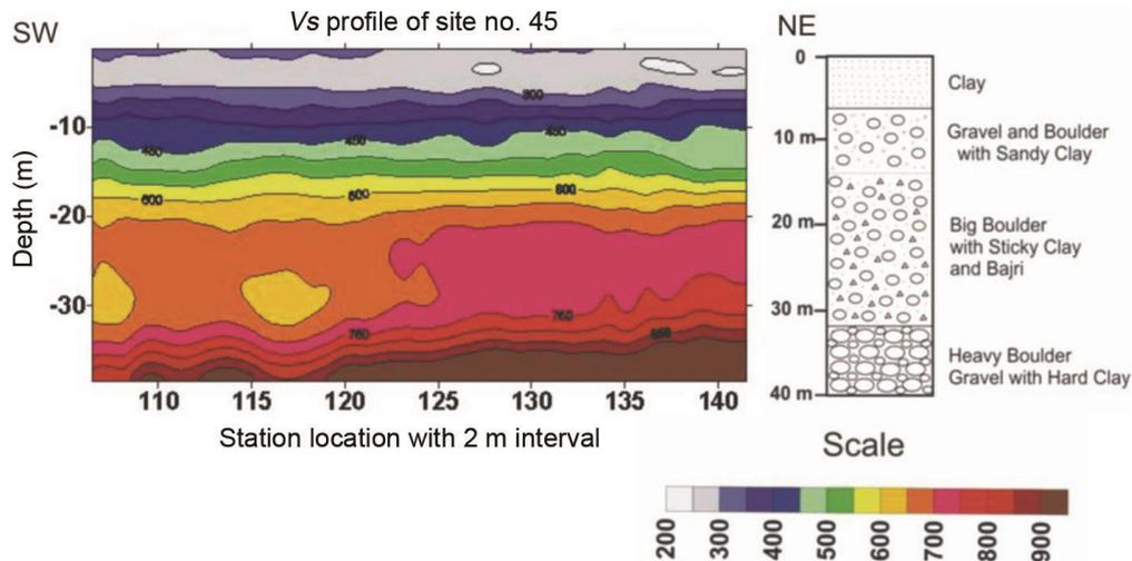
**Figure 9.** Shear wave velocity profile of Badripur site no. 46 (zone 5) showing different shear wave velocity bands ( $V_s$ ) with corresponding tube well log.
