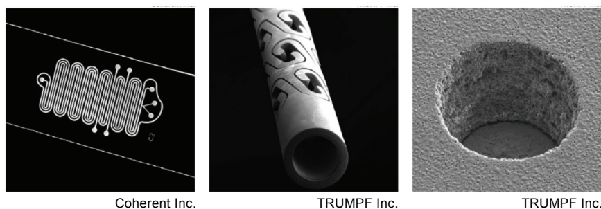
Figure 7. Femtosecond laser enabled engraving of micro-chip (left), precision patterns on metal alloys (centre) and micro-hole drilling in circuit boards (right). (Image taken from ref. 26.) CPA-based femtosecond lasers make the cleanest cuts.
