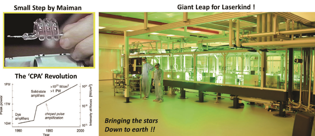
Figure 5. (Top left) A picture of the first ever laser unveiled on 16 May 1960 by Theodore H. Maiman at the Hughes Laboratories, USA. (Bottom left) Peak powers which were stranded till the 1980s at the gigawatt level in most labs around the world, got boosted by a factor of 100–1000 (1000 GW = 1 TW) almost immediately after CPA was invented. Today, the highest power available is at the petawatt (=1000 TW) level and these lasers use CPA. (Right) A portion of one of the biggest laser facilities in the world, at ELI Beamlines, Prague, Czech Republic.
