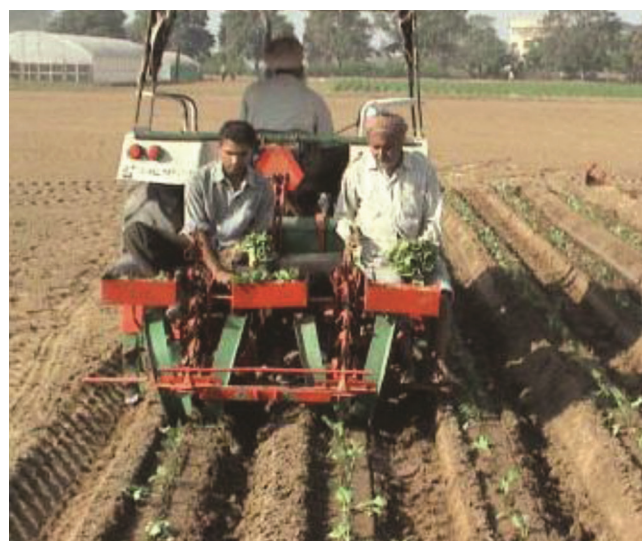
Figure 2. Pocket-type tractor drawn two-row semi-automatic vegetable transplanters 8 .
