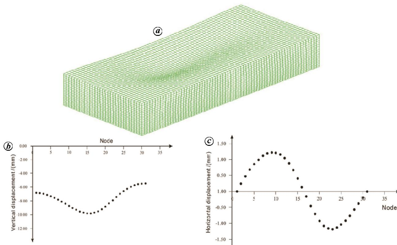
**Figure 4.** Displacements direction of ore body tendency. *a*, The mesh map and the shape of backfill in 3D simulation mode; *b*, Vertical displacement; *c*, Horizontal displacement.
