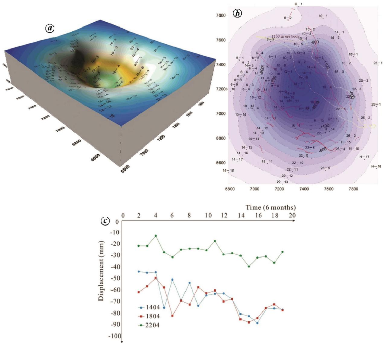
**Figure 3.** Ground subsidence of Jinchuan Mine. *a*, Ground subsidence in 3-dimension; *b*, Ground subsidence in 2-dimension; *c*, Vertical displacements of monitoring points on the backfill.
