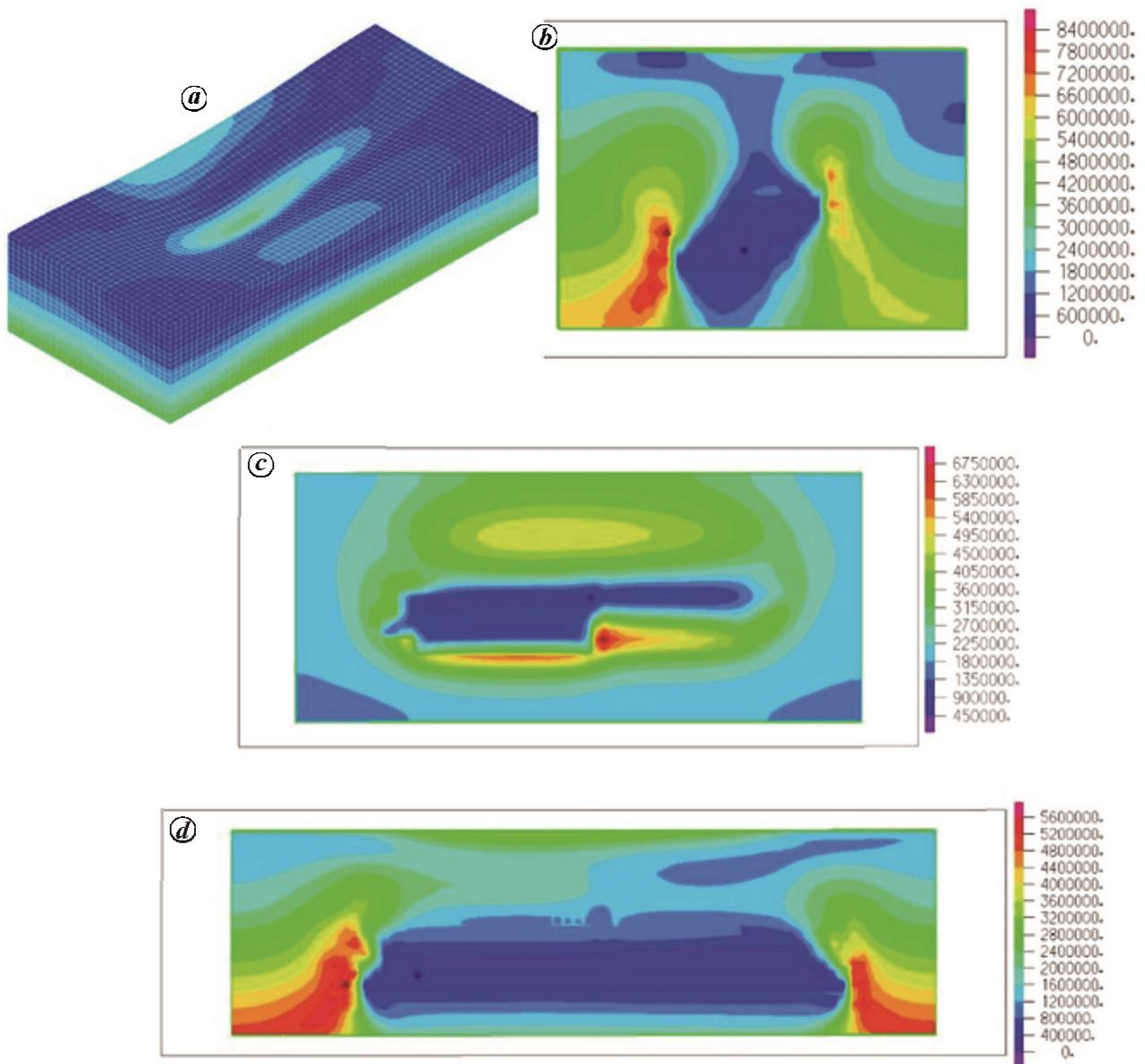
**Figure 5.** The shear stress distribution of model. *a*, Overall distribution of shear stress; *b*, The shear stress in direction of ore body tendency; *c*, The shear stress in direction of ore body deep; *d*, The shear stress in direction of ore body strike.
