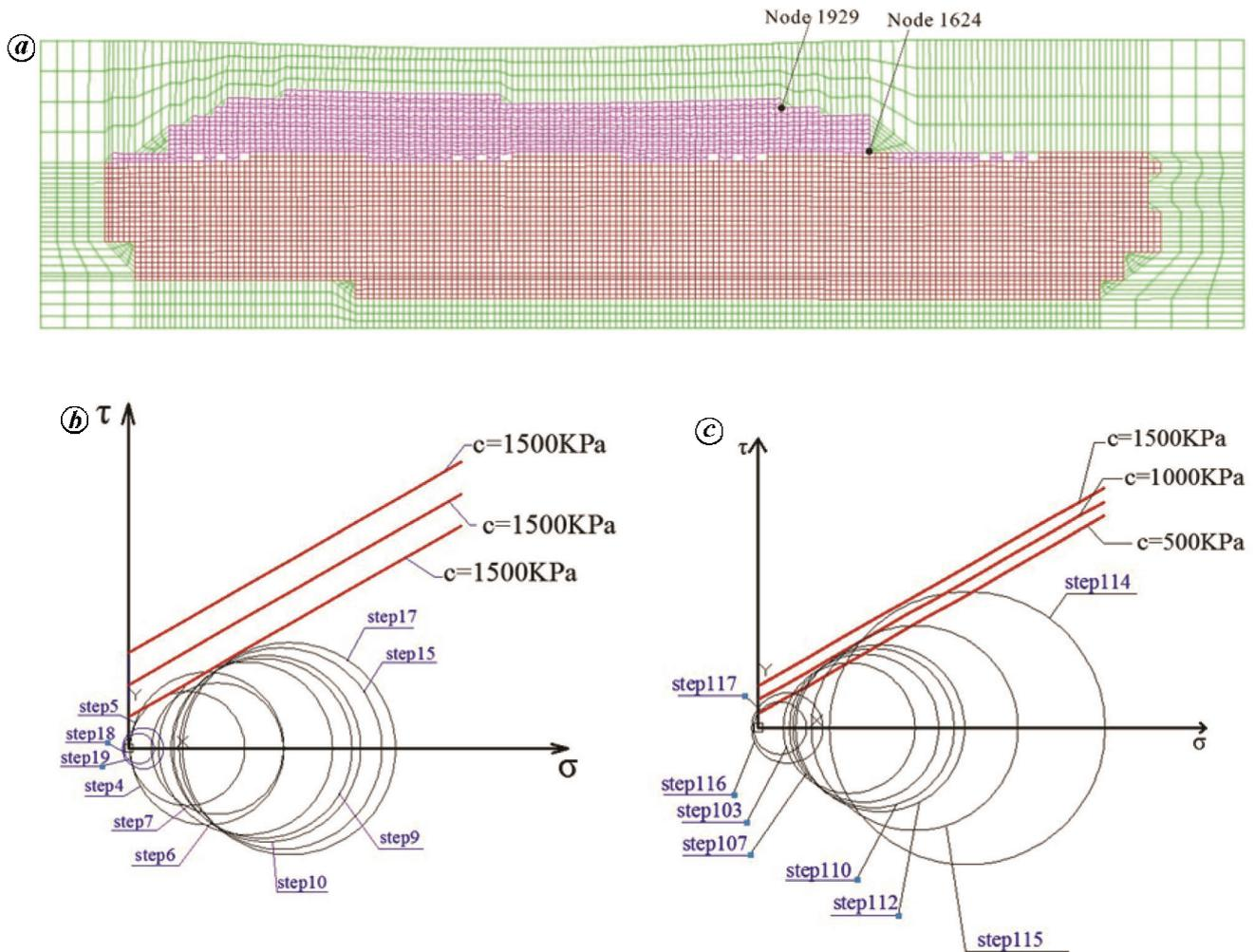
**Figure 6.** The Mohr's circle of special nodes of different excavation steps of 2-D numerical model. *a*, The mesh of 2D numerical model; *b*, The Mohr's circle of point 1929; *c*, The Mohr's circle of point 1624.
