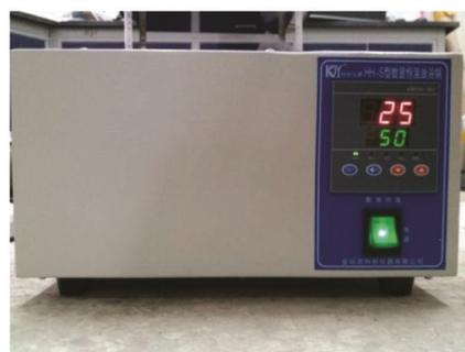
**Figure 2.** The thermostatic oil bath with digital display.
