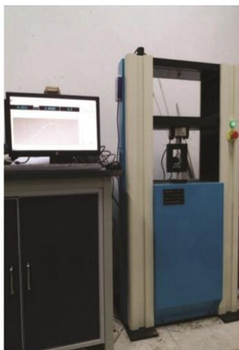
**Figure 3.** Rock indentation sclerometer under microprocessor control.
