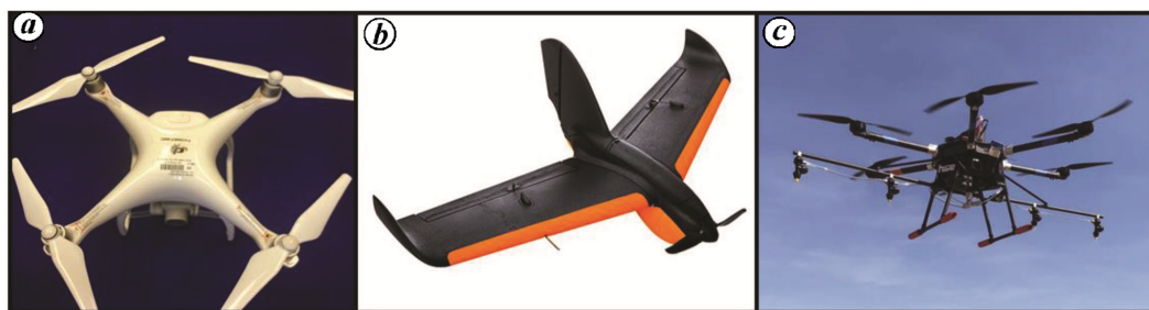
Figure 2. Notable UAV systems available in the market: (a) Rotary wing UAV (DJI Phantom 4), (b) Fixed Wing UAV (Sentera Phoenix 2) and (c) Spray UAV (HSE V6A).
