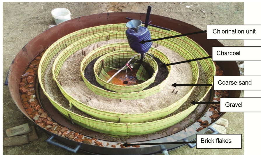
Figure 1. View of composite radial filter with filter medium and chlorination unit.
