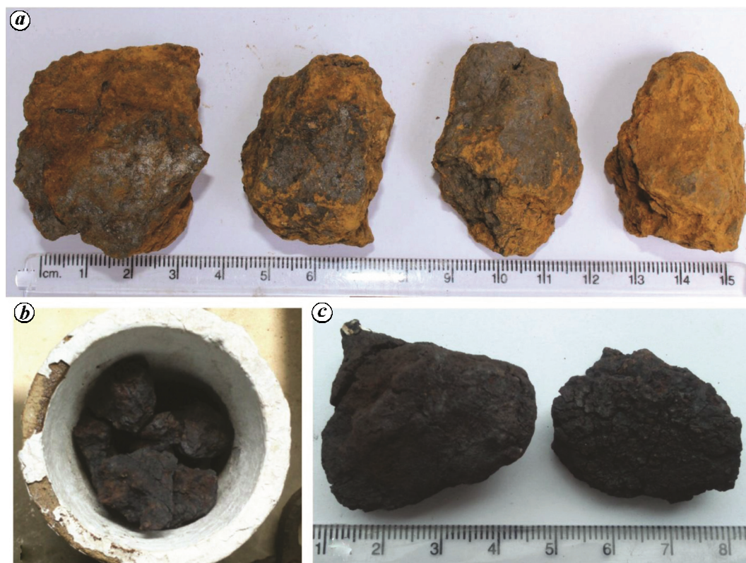
Figure 5. a , Material samples of bog iron ore from Malai Dai. b , Textural changes in iron ore (Malai Dai) in a furnace at 160°C. c , Textural changes in iron ore from Malai Dai in a furnace at 1200°C.
