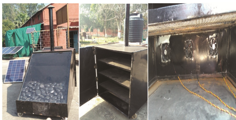
Figure 1. View of hybrid solar dryer, drying chamber and fans.
