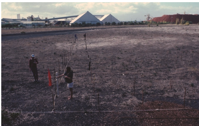
Figure 1. Transit poles mark grid lines for the combined magnetometer (operators' foreground) and metal detector survey (operators in the distance) at the Bunbury wrecks (B. Richards).
