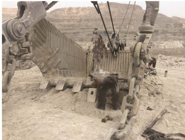
Figure 1. Dragline bucket teeth repair on site.
