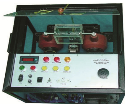
Figure 2. Schematic diagram of dielectric strength measuring equipment.
