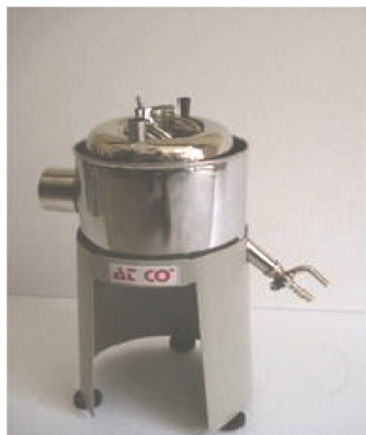
Figure 12. Schematic diagram of red wood viscometer.
