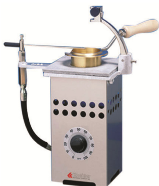
Figure 8. Schematic diagram of Cleveland open cup flash point tester.
