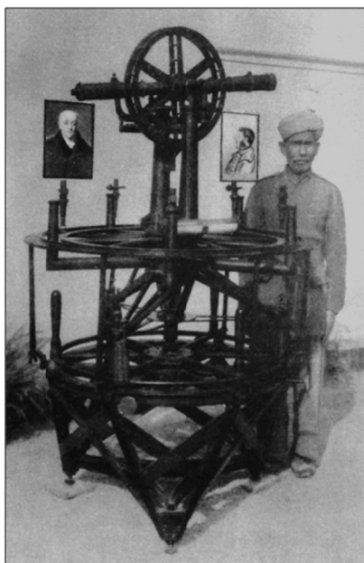
Figure 5. The great Cary theodolite with a 36” azimuth circle used by William Lambton. [Source: Philimore 34 , plate 6, between pp. 94 and 95]. The legend supplied by Philimore 34 : ‘The William Cary great theodolite used by Lambton and his assistants 1802–1822, and by Everest 1823–1825, reconstructed by Henry Barlow in Calcutta 1831–1834, and from 1835 to 1866 in constant use. Now standing in Survey Museum in Dehra Dun’. [Note: Lambton’s portrait in the background.]
