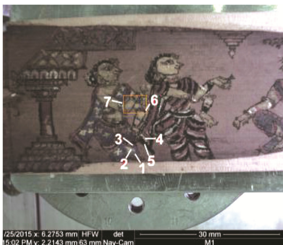
Figure 5. Photograph of illustrated palm leaf manuscript using navigation camera in the SEM chamber. (Measuring points for pigments: 1, blue; 2, yellow; 3, red; 4, white; 5, blue.)
