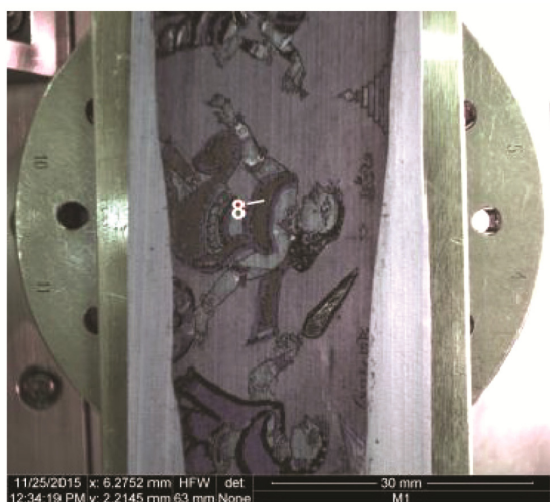
Figure 7. Photograph of illustrated palm leaf manuscript using navigation camera in the SEM chamber (measuring points for green pigment 8).
