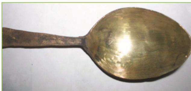
Figure 4. The kitchen spoon reconstructed at Khagra: after final finishing became the drawn cup 80 mm long, 50 mm wide and 16 mm deep with an average thickness of \sim 1.0 mm.
