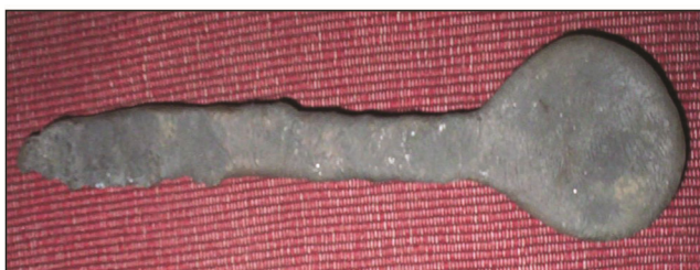
Figure 3. Cast ingot of high-tin bronze having chunky sections of elliptical disc and triangular-shaped handle.
