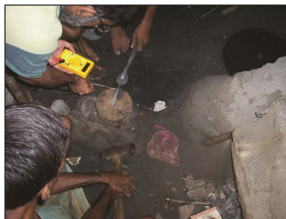
Figure 2. Experimentation at Khagra, Murshidabad district, West Bengal (WB) (measuring temperature of the hot blank) at the site of the forging shed.
