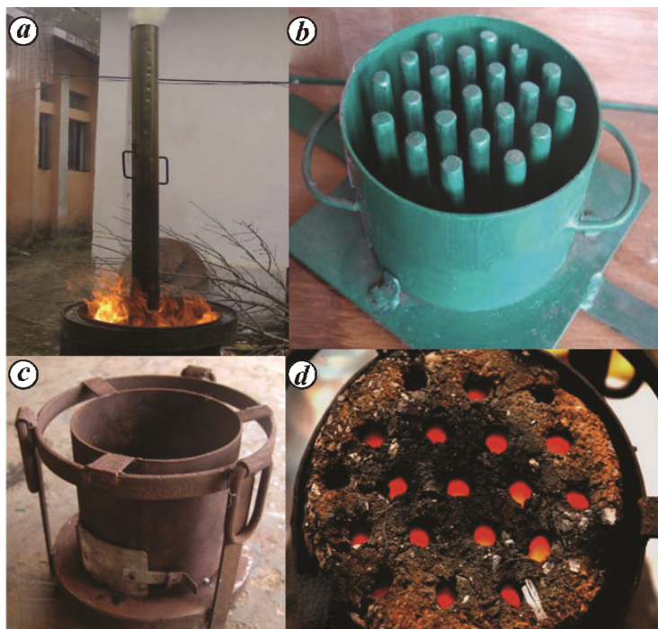
Figure 1. a , A 200 l oil container charring drum; b , beehive briquetting mould; c , metallic stove; d , burning beehive briquette.
