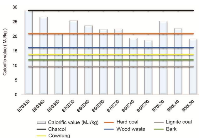
**Figure 4.** Comparison of calorific value of biochar blocks with different fuels.
