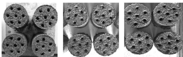
**Figure 3.** Pine needle biochar blocks produced by manually operated block-making machine.
