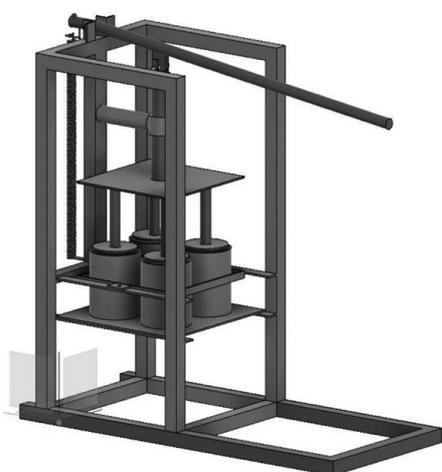
Figure 1. Manually operated block-making machine.
