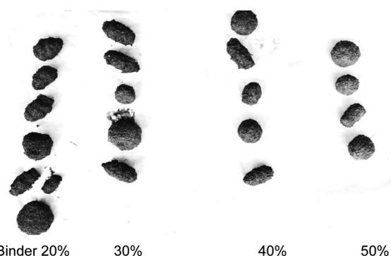
Figure 2. Composition of biochar and binders in different ratios.
