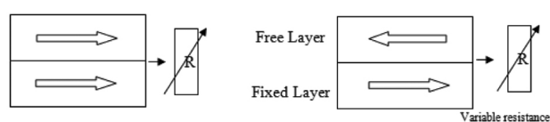
Figure 2. Resistive element from MTJ.
