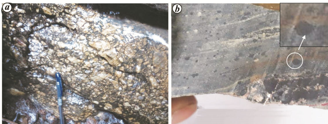
Figure 2. Field photographs of Laggi Gamlin area showing ( a ) uraniferous brecciated marble of Laggi Gamlin-1 uranium mineralization, and ( b ) sheared magnetite grain and uraniferous magnetite-bearing quartzofeldspathic vein in sheared magnetite quartzite of Laggi Gamlin-2 uranium mineralization.
