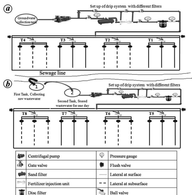
**Figure 2.** Layout of the experiment under different treatments. *a*, Groundwater applied for treatments T1 to T4. *b*, Wastewater applied for treatments T5–T8. Two separate set-ups of drip irrigation system were installed for groundwater and wastewater application.
