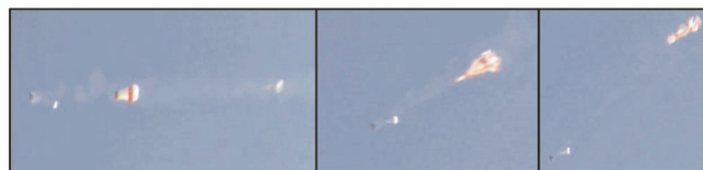
Figure 3. Main parachute failure due to high snatch force.
