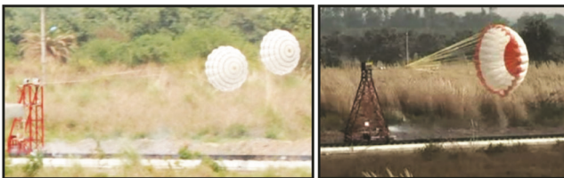
Figure 7. Rail track rocket sled tests for pilot and drogue parachutes.
