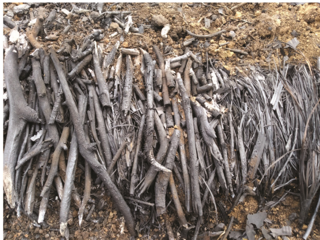
Figure 4. Biochar prepared from grasses and small branches during oxygen-limited burning in raised beds.
