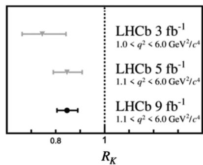
**Figure 2.** Summary of the LHCb measurements of  $R_K$ . The numbers 3, 5, 9  $\text{fb}^{-1}$  indicate the amount of data collected and the dotted vertical line is the SM expectation. The quantity  $q^2$  refers to the square of the Lorentz-invariant mass of the two leptons in the final state. The bottom-most experimental number is the most recent measurement.
