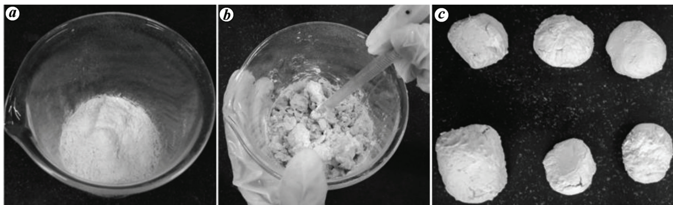
Figure 1. Steps followed in the process of poulticing. a , Cellulose powder in dry form. b , Mixing of cellulose powder with water to prepare the poultice. c , Samples covered with cellulose poultice left for drying.
