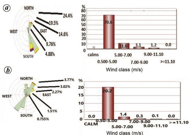
**Figure 9.** Direction and wind class diagrams at (a) Lavasan station and (b) at the Shemiran station.
