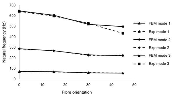
**Figure 9.** Variation in vibration frequencies of simply-supported LCB for different fibre angles.
