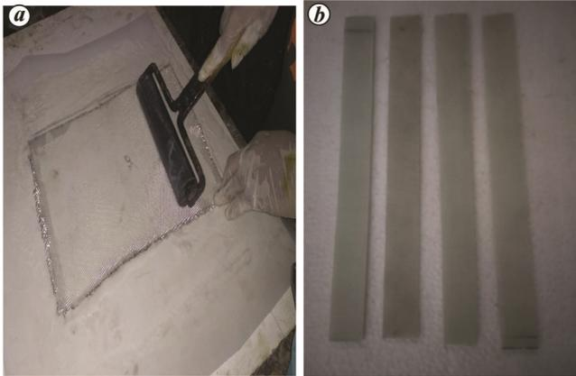
**Figure 3.** LCB fabrication: (a) hand lay-up and (b) produced beam samples.
