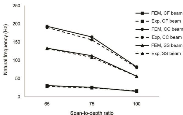
Figure 10. Variation in first-mode frequency with respect to  $L/h$  ratio for LCB with 0° fibre orientation.
