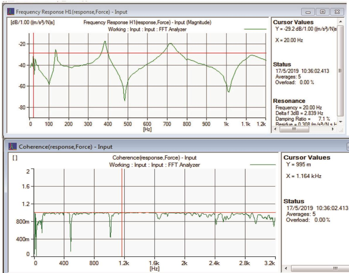
Figure 6. Frequency response functions and coherence graph for clamped-free beam with 0° fibre orientation.
