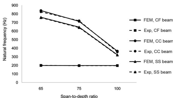
Figure 12. Variation in third-mode frequency with respect to  $L/h$  ratio for LCB with 0° fibre orientation.
