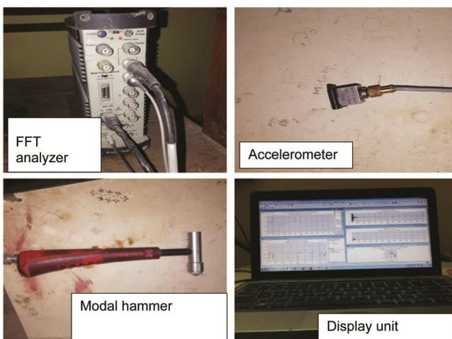
**Figure 5.** Complete experimental set-up.
