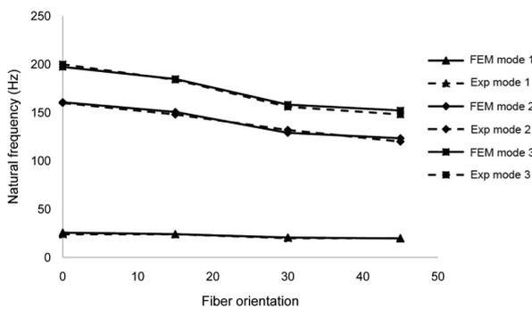
**Figure 7.** Variation in vibration frequencies of cantilever LCB for different fibre angles.
