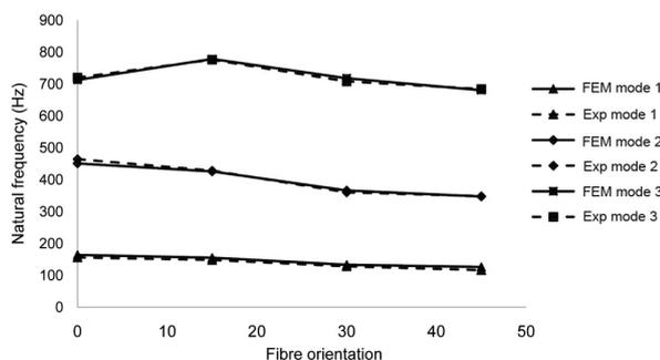
**Figure 8.** Variation in vibration frequencies of fixed LCB for different fibre angles.
