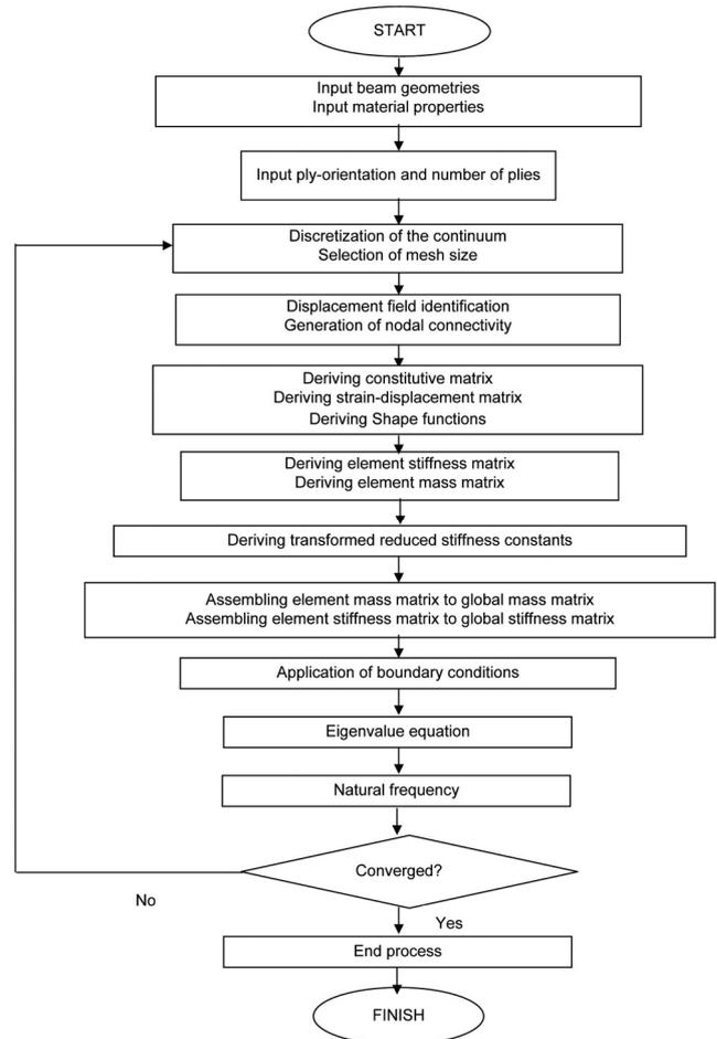
**Figure 2.** Flow chart of MATLAB program for free vibration of LCB.
