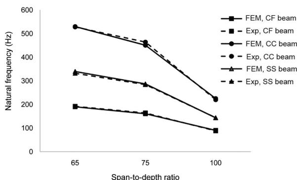
Figure 11. Variation in second-mode frequency with respect to  $L/h$  ratio for LCB with 0° fibre orientation.
