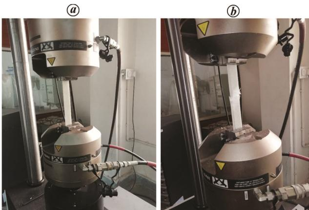
**Figure 4.** Tensile testing of glass/epoxy LCB in INSTRON 8862: (a) specimen before failure and (b) specimen after failure.
