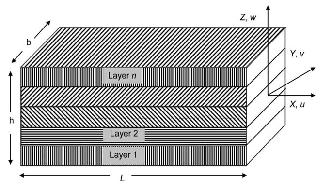
Figure 1. Geometry of laminated composite beam (LCB).
