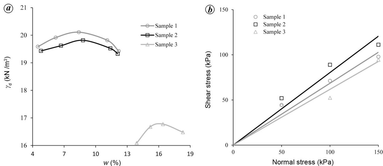
Figure 2. (a) Compaction and (b) shear strength characteristics of dump materials.
