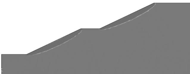
**Figure 6.** Typical failure pattern obtained from dump slope analysis based on a laboratory study ( $\alpha_d = 30^\circ$ ).
