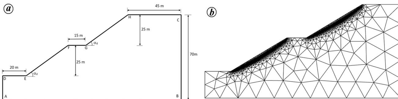
**Figure 4.** Details of dump slope: (a) soil domain and (b) mesh details for the analysis of dump slope.
