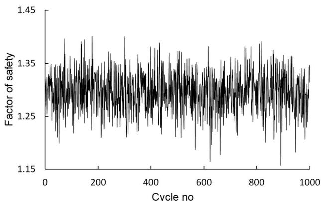
Figure 9. Variation of factor of safety over 1000 cycles.
