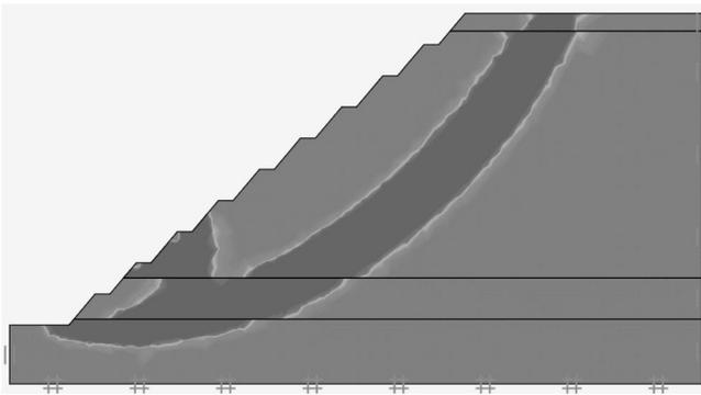
**Figure 11.** Failure pattern obtained at the end of 1000 cycles for highwall slope.
