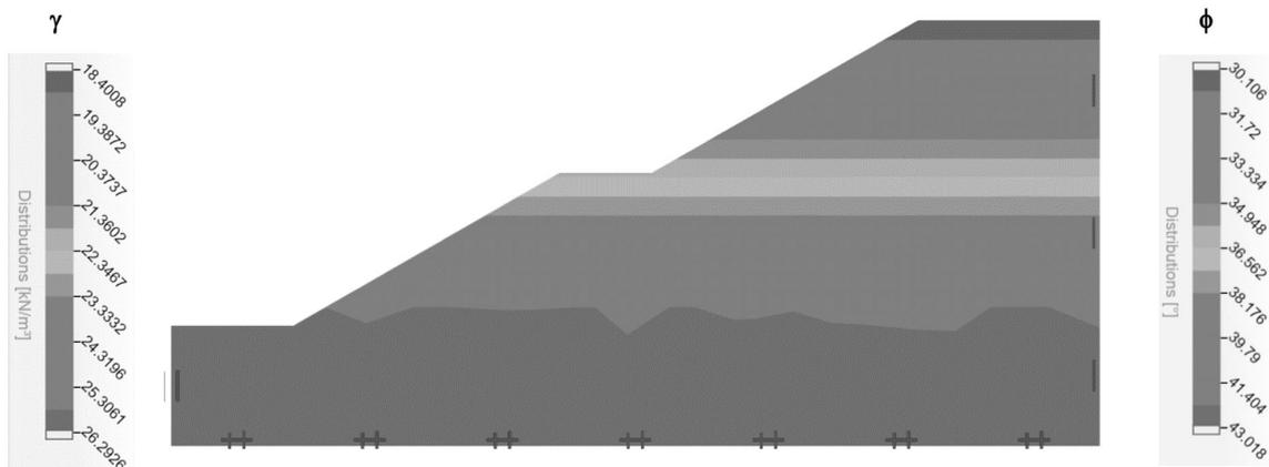
Figure 7. Variation of friction angle and unit weight in the soil domain based on shear wave velocity profile.
