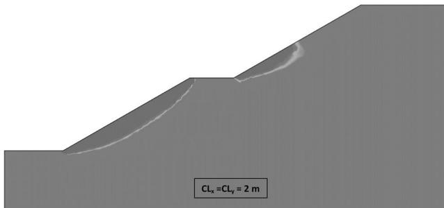
**Figure 10.** Failure pattern obtained at the end of 1000 cycles for dump slope.
