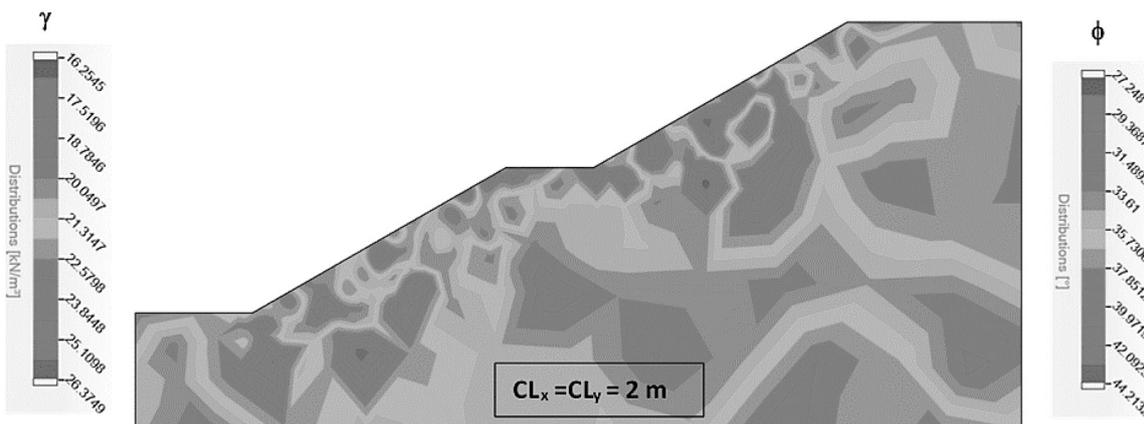
Figure 8. Variation of unit weight and friction angle in the domain for probabilistic analysis.
