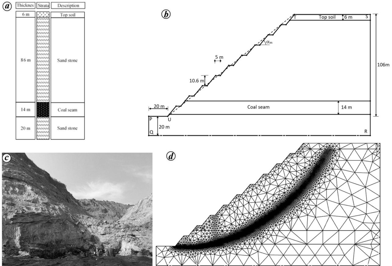
**Figure 5.** Details of highwall: (a) typical layer profile, (b) soil domain, (c) photograph of a highwall slope and (d) mesh details for the analysis of highwall slope.
