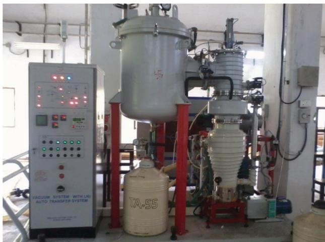
Figure 10. High vacuum induction furnace.
