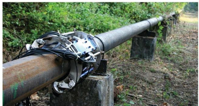
Figure 17. EPIG tool for 6" NB pipe inspection.
