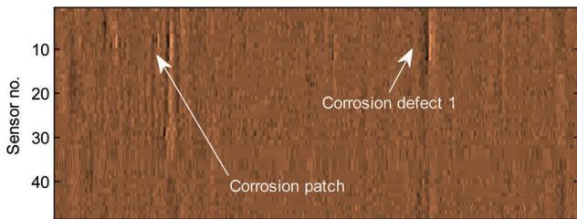
Figure 19. C scan showing corrosion patch and isolated defect of fire water line.
