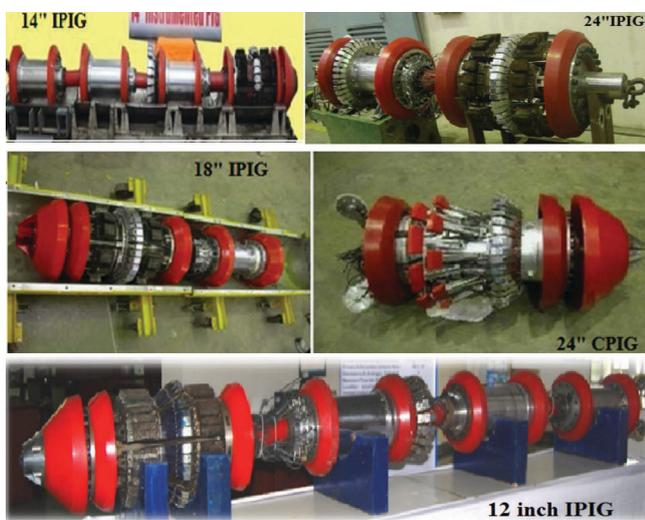
Figure 15. Different sizes of indigenously developed ILI tools.
