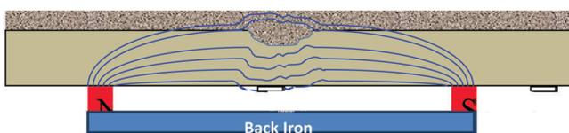
Figure 1. Schematic view of the MFL principle.
