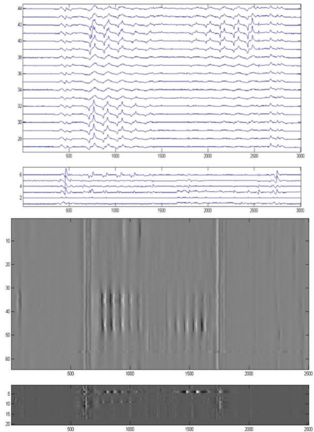
Figure 20. Internal defects detected by MFL and eddy current sensors.
