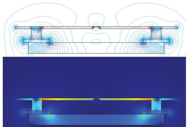
Figure 2. Finite element analysis of the magnetizer unit.
