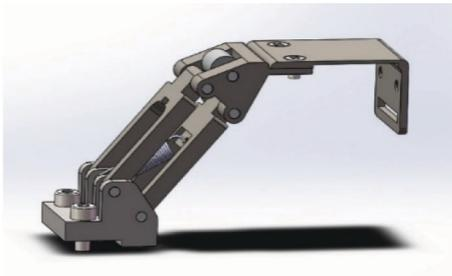
Figure 4. Sensor carriage.
