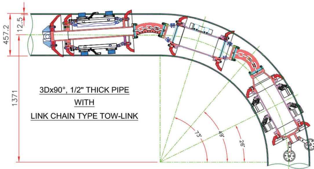
Figure 8. Three-dimensional bend negotiability of IPIG.
