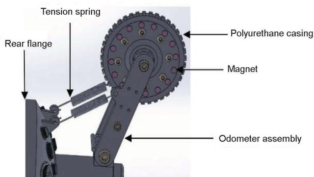
Figure 6. Odometer system.
