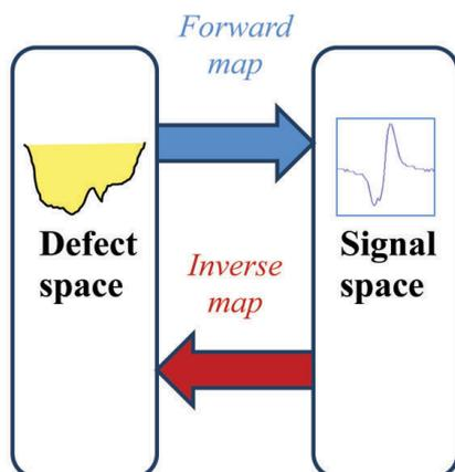
Figure 10. Forward and inverse mapping for defect characterization.
