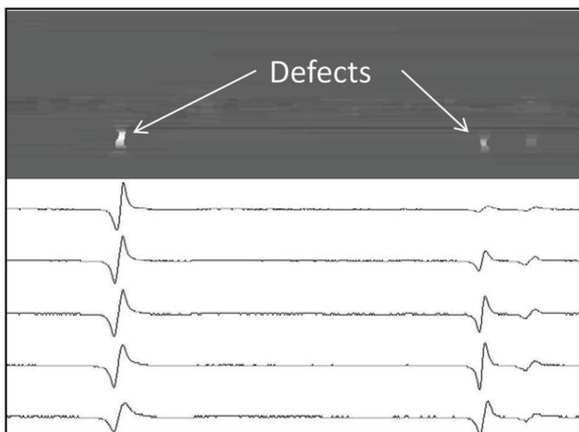
Figure 9. Surface image of a pipeline showing defects.
