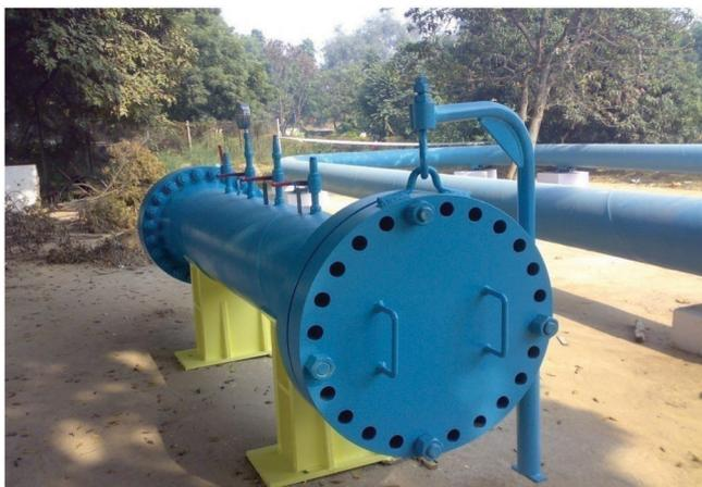
Figure 11. Rig for pressure testing of modules.
