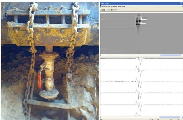
Figure 16. Pilferage points detected by IPIG.
