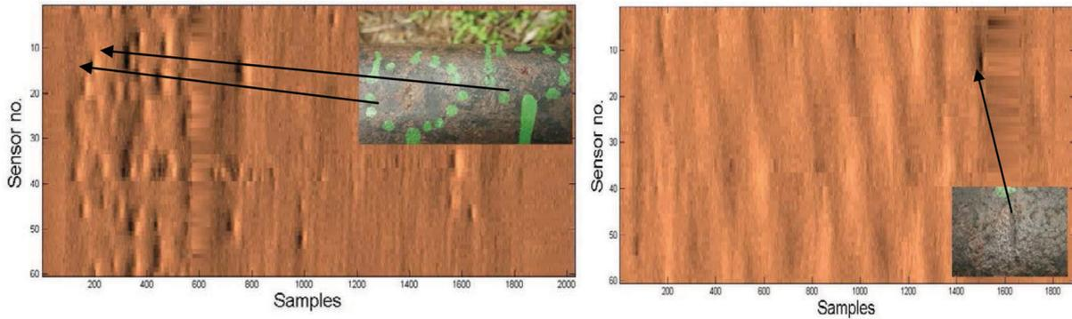
Figure 18. C scan and actual defects of pipeline at IF3.
