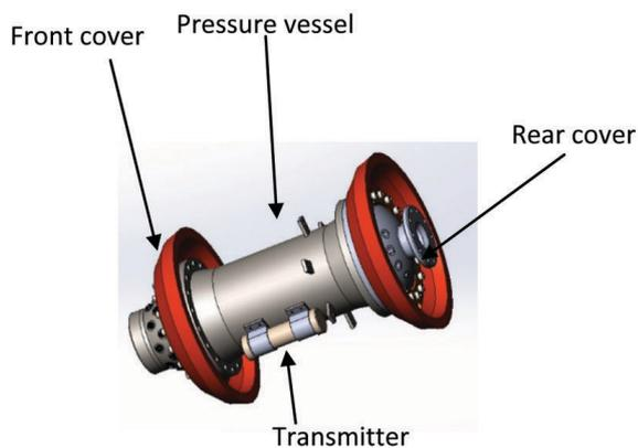
Figure 5. Data acquisition system-cum-power supply module.
