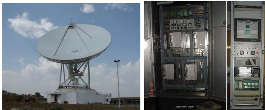
Figure 12. IDSN32 antenna with servo cabinets.
