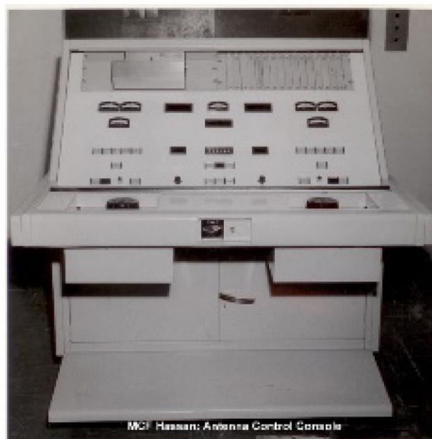
**Figure 5.** Antenna control console for MCF Hassan.
