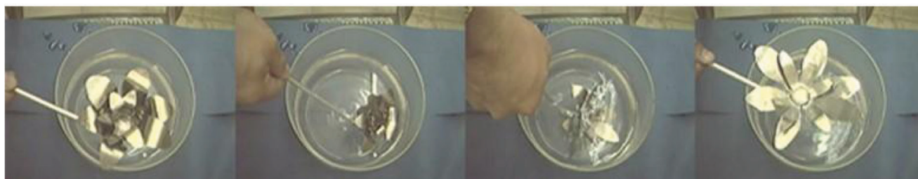
Figure 1. A 'flower' fabricated from thin sheets of equiatomic Ni-Ti alloy is used to demonstrate the shape memory phenomenon. The flower, which is easily deformed into a 'bud' at ambient temperature, rapidly 'blossoms' or recovers its original shape (and dimensions) on raising the temperature by immersing it into a bowl of hot water.
