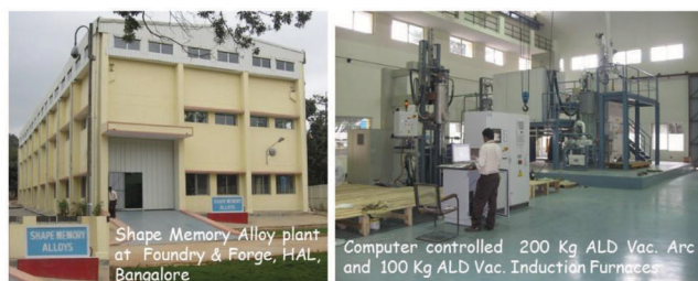
Figure 14. SMA manufacturing facility set up at F&F, HAL, Bengaluru, under a tripartite MoU between BARC, ADA and HAL for the transfer of technology of Ni–Ti SMAs and Ni–Ti–Fe heat-shrinkable ferrules.
