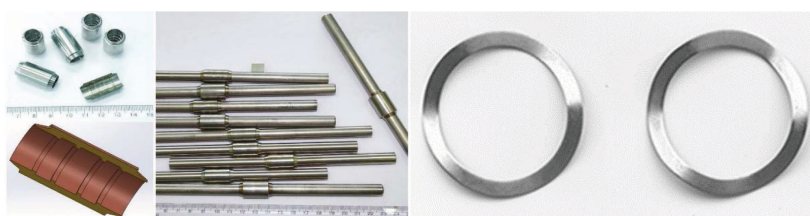
Figure 5. Superelastic Ni–Ti SMA three-wave springs and Ni–Ti–Fe heat-shrinkable couplings developed for aerospace applications.
