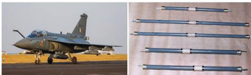
Figure 4. Ni–Ti–Fe shape memory alloy (SMA) heat-shrinkable ferrules developed by BARC, Mumbai, have been deployed for application in the Tejas light combat aircraft (LCA).
