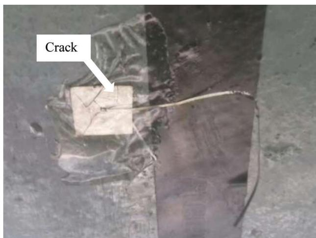
**Figure 20.** Close up of broken PZT patch bonded to the girder.
