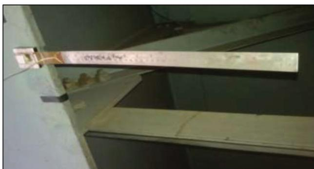
**Figure 17.** PCH with MFC piezo patch attached underneath the steel girder.
