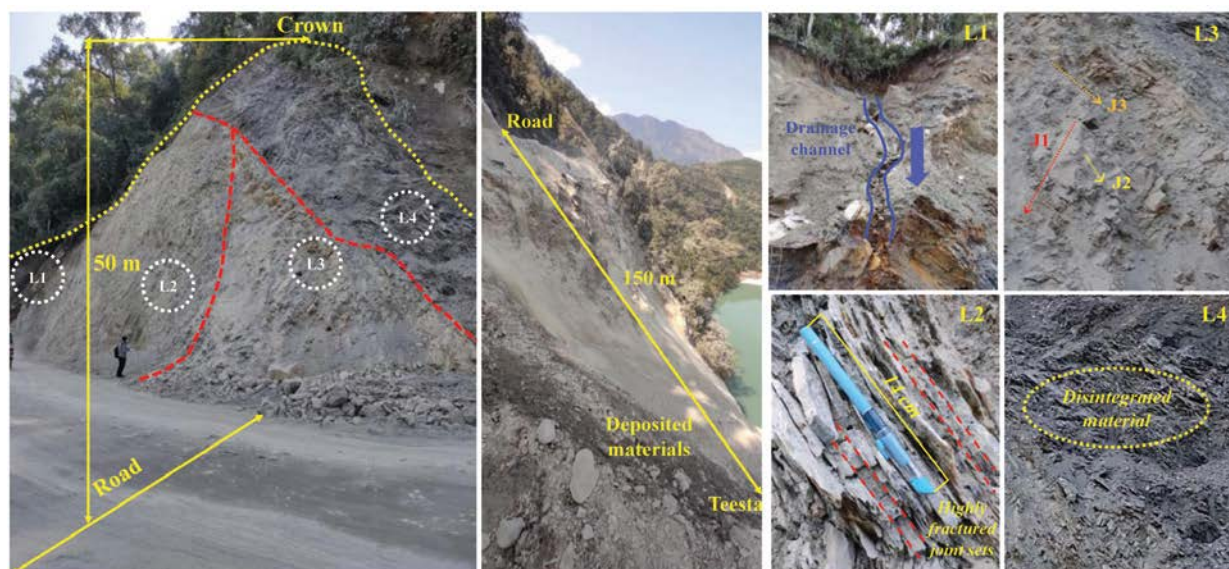
Figure 3. Field photographs of Birik Dara landslide. L1–L4 represent locations from where rock samples were collected for laboratory testing.
