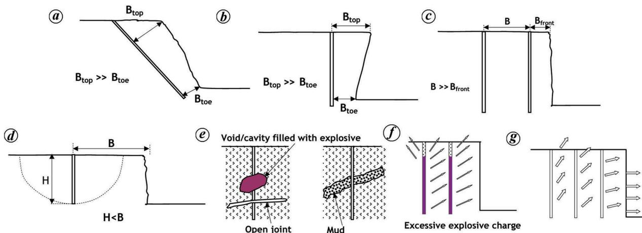
**Figure 8.** Common causes of flyrock in surface bench blasting. *a*, Incline hole causing less toe burden. *b*, Under-confined at the toe. *c*, Too less front burden. *d*, Too large front burden. *e*, Cavity, open joint and mud seam. *f*, Excessive charge and very small top stemming. *g*, Inadequate delay timing (back rows).
