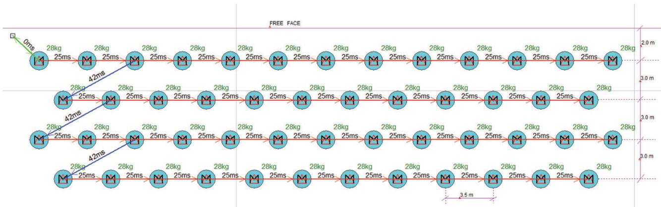
Figure 16. Suggested surface firing pattern of holes for the blasting zone beyond 300 m.
