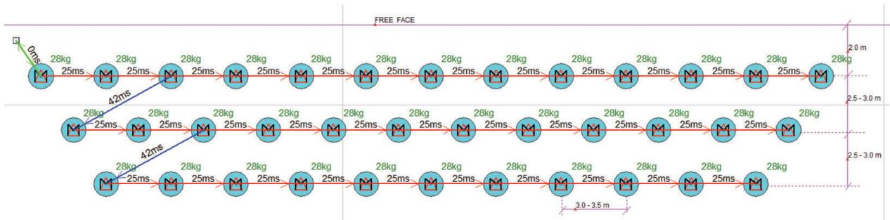
Figure 14. Suggested surface firing pattern of holes for blasting zone of 200–300 m.
