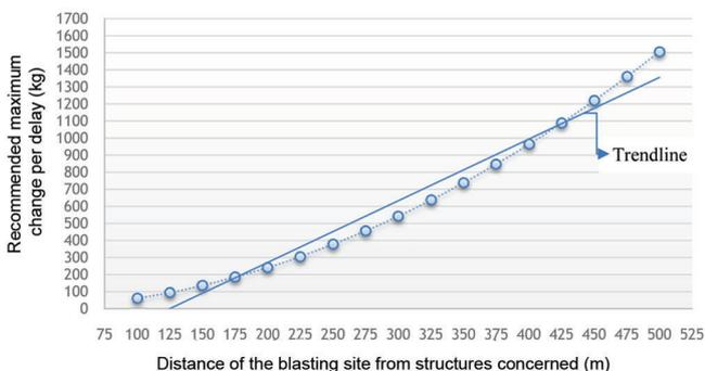
**Figure 10.** Safe maximum charge per delay to be fired in a round of blast.
