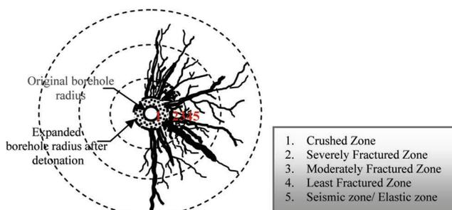
Figure 1. Different zones of rock deformation around a blasthole<sup>5</sup>.
