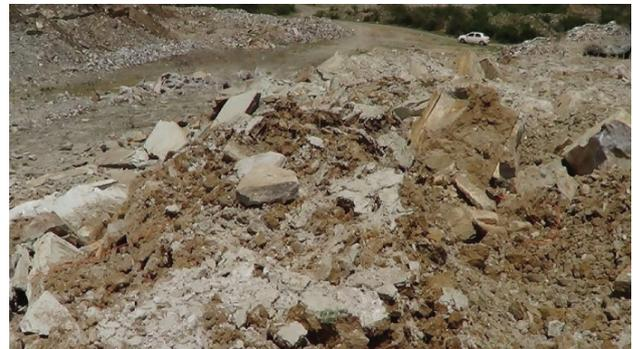
**Figure 13.** Blast fragmentation of quarry no. 5.
