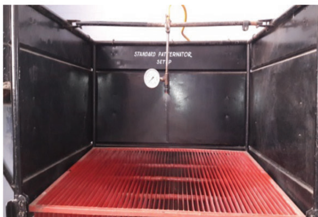
Figure 2. Calibration of urea spraying nozzles on a pattenator.
