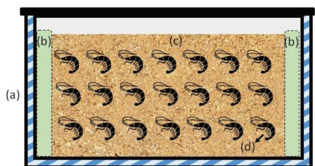
**Figure 3.** Schematic representation of waterless system for live fish transportation. a, Insulated container with lid; b, cooling unit; c, pre-chilled layering medium; d, live fish/shellfish.
