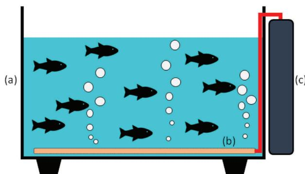
**Figure 2.** Schematic representation of open system for live fish transportation. a, Container; b, oxygen diffuser; c, external oxygen source.
