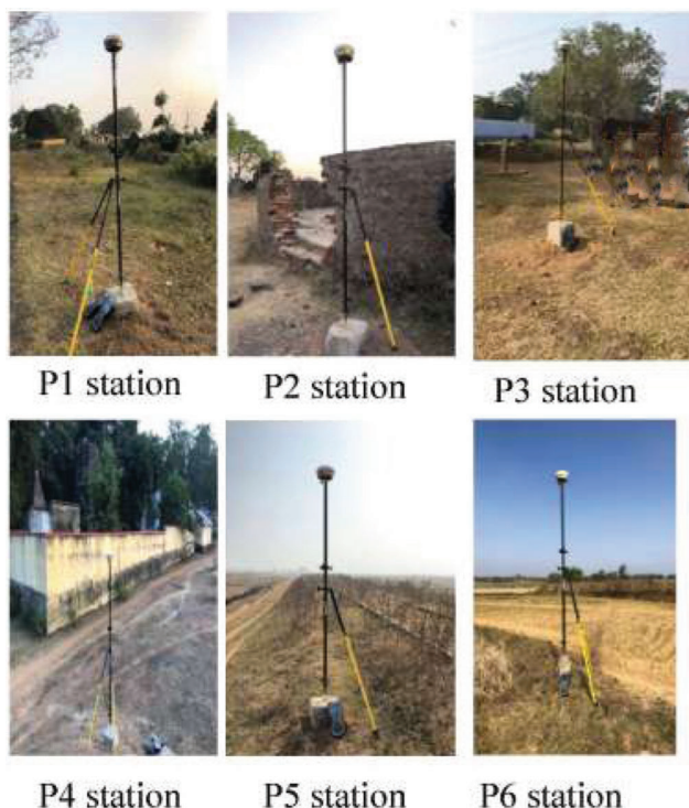
Figure 4. Primary control points at Kasta East Coal Block.
