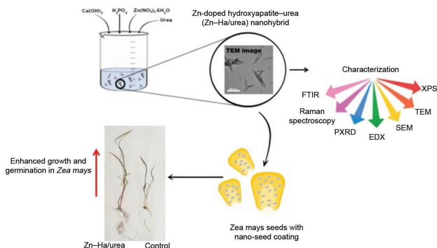
**Figure 1.** Graphical representation of synthesis and characterization of Zn-doped HA-urea nanohybrid and its use in enhanced germination and seedling growth.
