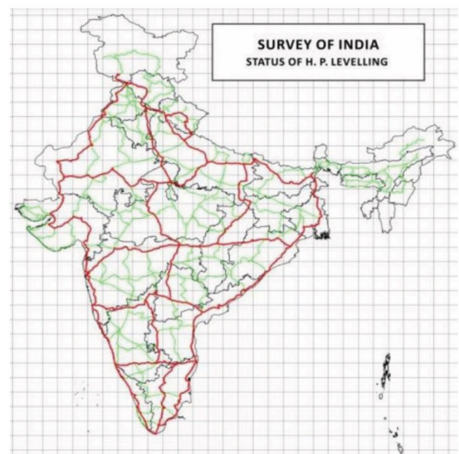
Figure 3. Levelling net for IVD2009 (red line shows primary network). (Source: ref. 19).
