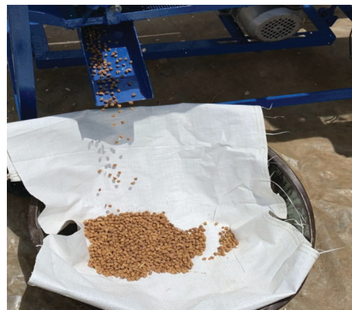
Figure 1. Threshing of chickpea seeds using solar operated plot thresher.
