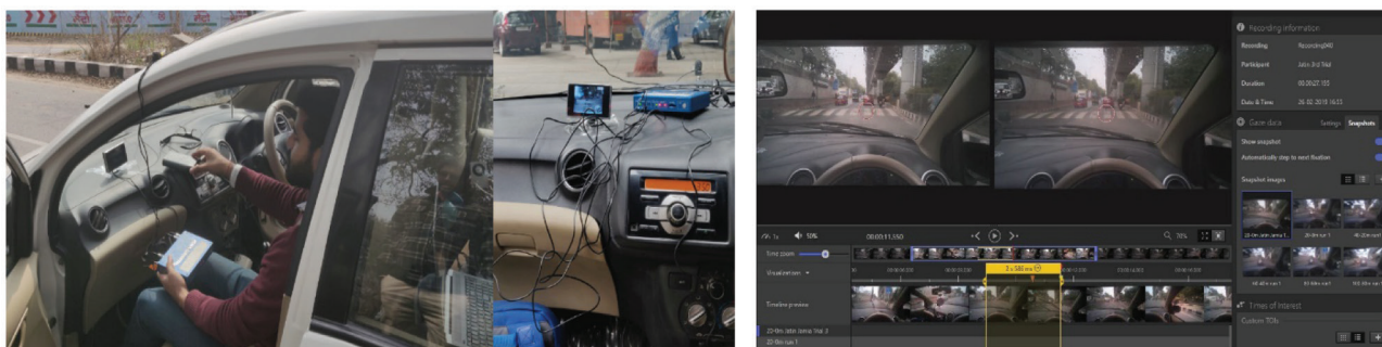
Figure 2. Set-up of V-box and eye-tracker software with timeline data series.
