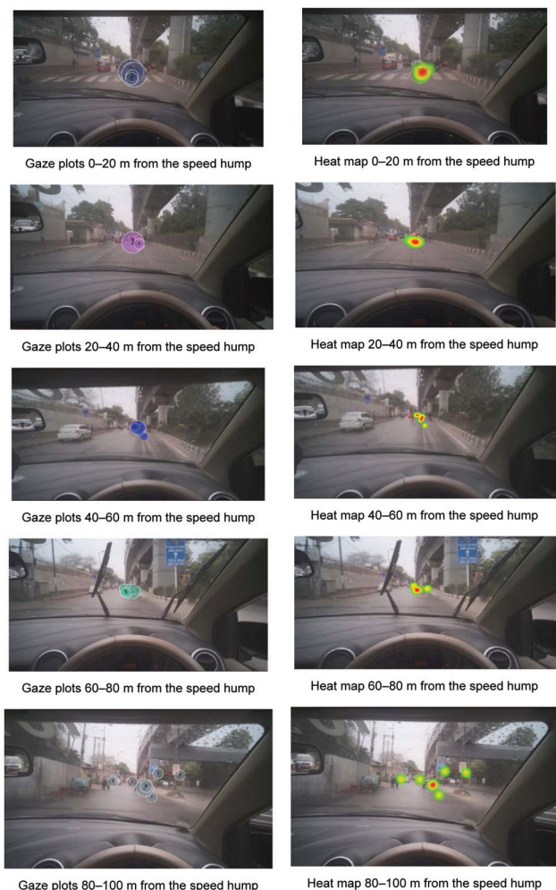
Figure 5. Gaze plots and heat map of a driver approaching a speed hump.
