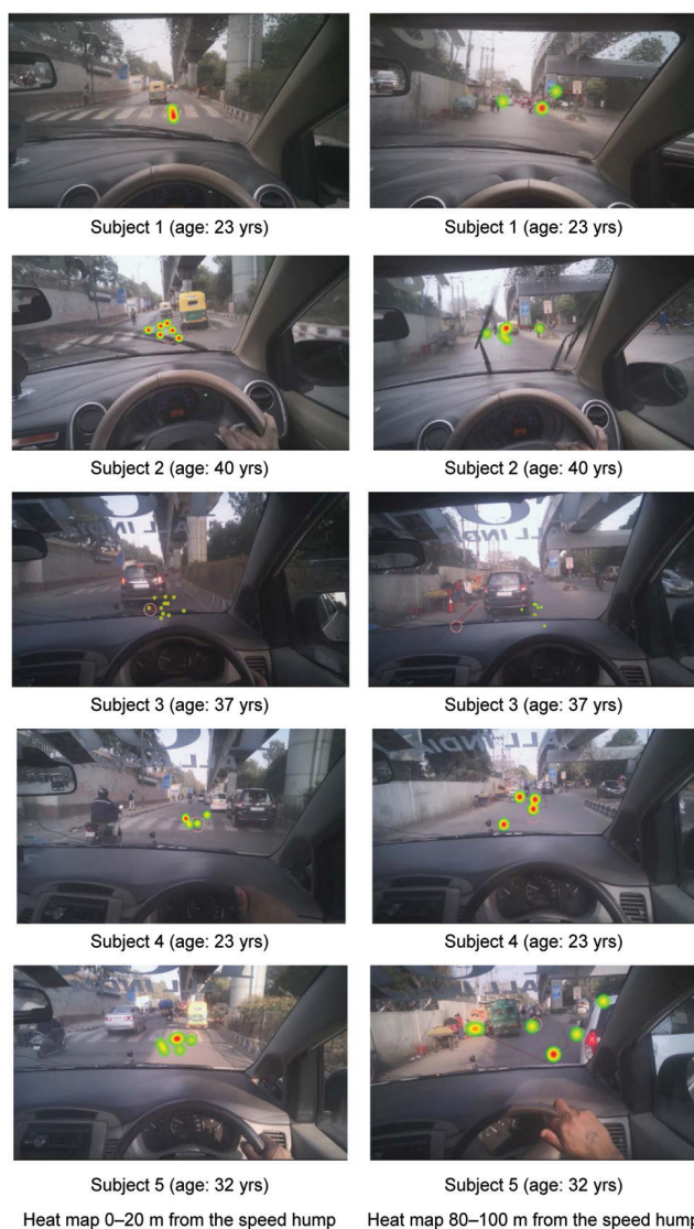
Figure 6. Heat map of drivers of different age groups approaching a speed hump.
