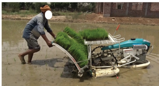
Figure 1. View of the walk-behind-type paddy transplanter in operation.
