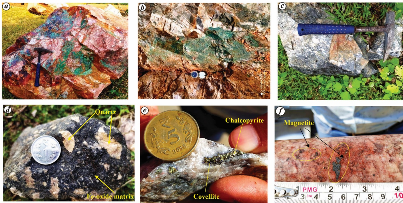
Figure 2. Field photographs showing surface indications of mineralization and associated alteration. a , Malachite stains and iron leaching in quartz vein. b , Chloritic-argillic alteration and malachite-iron stains in quartz vein. c , Iron oxide-rich matrix-dominated hydrothermal breccia. d , Hand specimen of hydrothermal breccia showing sub-rounded to angular quartz fragments in the iron oxide matrix in a closer view. e , Clustered grains of Cu sulphide with probable gold. f , Drill-core sample showing magnetite as dissemination and fracture filling in silicified zones within porphyritic granites away (around 60 m) from the ore zone.
