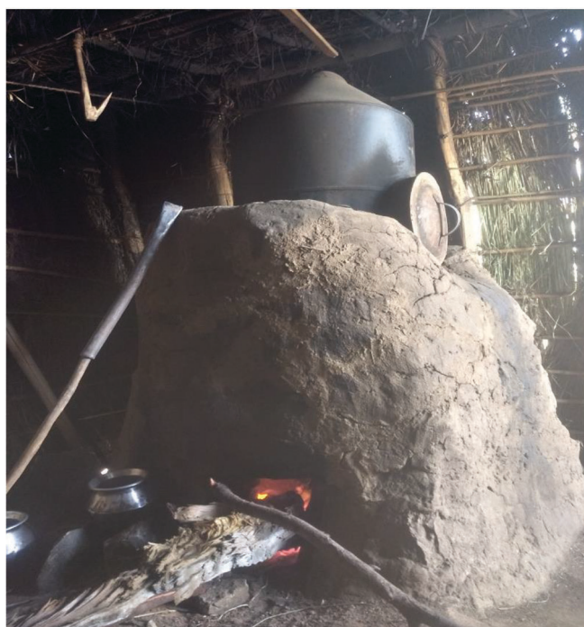
Figure 4. Primitive or old type of distillation unit used by the tribal farmers for the distillation process.
