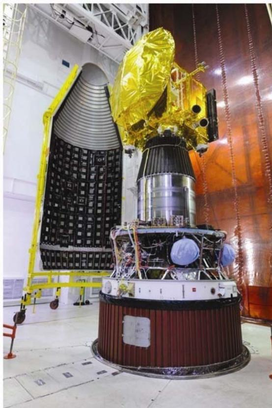
Figure 3. Mars Orbiter integrated to PSLV-C25.
