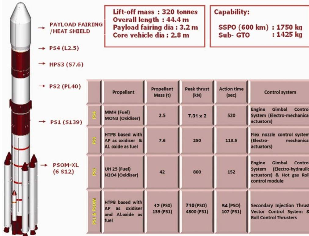
Figure 2. Configuration of propulsion stages in PSLV-XL.
